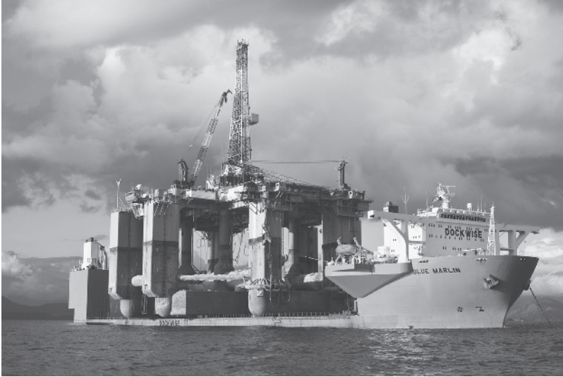
FIGURE 1.1 Complex systems: The heavy-lift ship MV Blue Marlin transporting the 36,000 metric ton drilling platform SSV Victoria . (Source: Dockwise/Rex Features/Associated Press)
